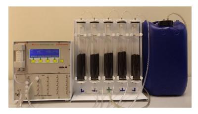
Additional T pieces can be added to the buffer volume tubing, to connect to further sets of sample columns in the same way. The other option is to use one buffer volume per rack, if you have the space, to ensure an even flow of air to each rack.
