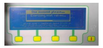
The analyser is cycling through all of the 'inlet valves' for only around 10 seconds each. Allow the instrument to finish this process, then the menu screen will appear again.
