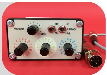
For independent, flexible control of the ADC White and RGB LED light units (released 2018)
