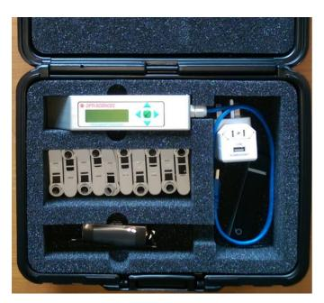
The Fv/Fm meter is supplied in a rigid, clam shell case which also holds the travel charger, battery, 10 dark adaption clips, charging lead and manual on a USB stick.
