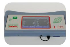
The LCi T provides unlimited data storage. All experimental protocols, data and calculations are stored on Secure Digital (SD) cards. SD cards can be interchanged for individual users or for specific experimental applications.
