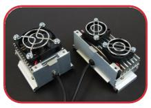
A micro PAR sensor measures the light emitted from a fitted LED array, onto the leaf surface. The light units closely replicate the PAR spectrum evenly throughout the leaf chamber window.
