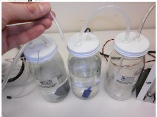
When the pump is switched off the glass jars will be lightly pressurised which will normally result in water flowing backwards up the pipes. To prevent this, simply remove both pipes from the first water bubbler as soon as the pump is switched off, as shown opposite.
