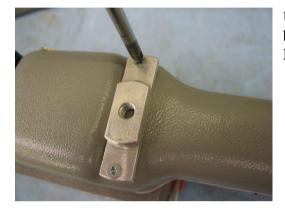
Unscrew the two retaining screws from the tripod boss.
