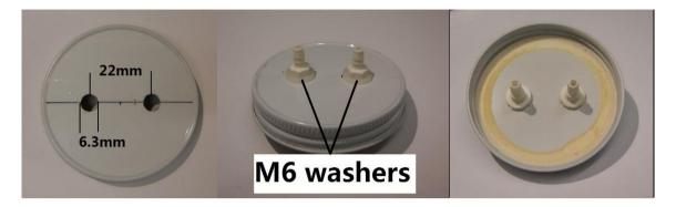
Next apply some two part glue using a cocktail stick to make a seal around the bulkhead connectors on both sides of the lid as shown below.
