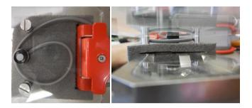
7. Fit the radiation shield as shown above, taking care not to trap the PAR cable.
