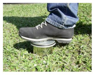
This minimises gas transference through the soil and also to provide more support to the Soil pot. Firmer soil may be difficult to penetrate and the "Collar insertion pad" should be used (see image above).
