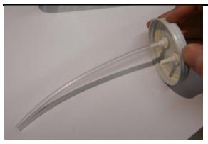
Connect this length of tubing to one of the bulkhead connectors on the inside of the lid (see left). If this buffer is connected to a console then the console "air in" entry connects to the buffer entry without the long tube on it, the "short" air entry.
