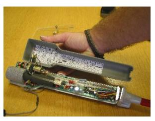
If you wish to completely remove the handle cover, take a note of the orientation of the connectors (there is a diagram inside the handle cover) and unplug the two sockets of the Tleaf thermistor and the CO<sub>2</sub> zero potentiometer wires from the PCB.
