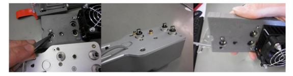
3. Remove the lower jaw and retrieve any O rings that have come off with the jaw, using a pair of blunt tweezers. Take care not to damage the O rings.
