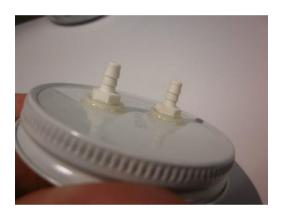
Next apply a few turns of PTFE tape to the glass thread on the jar, be sure to apply in the direction as shown (clockwise) so that the lid screws on with the same direction as the tape (see below left). Before screwing on the lid, cut a 3 mm bore length of tubing to length of the jar minus 20mm (see below right).
