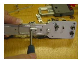
Unscrew and remove the two screws from the lever catch body.
