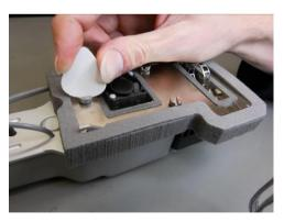
Tighten the screw <u>until the tool just starts to bend</u> and then stop.
