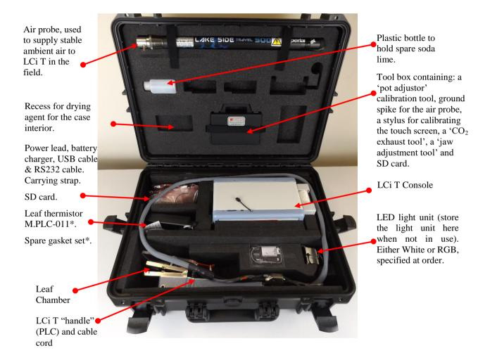
**NOTE** the cord must be stored in exactly this way.
