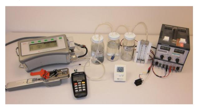
Before powering up the pump (shown above connected to a variable power supply), check that the water temperature is slightly cooler than ambient conditions, power up the pump at a flowrate of 500ml/min. Carefully watch the pipework coming out of the bubbler system and make sure no condensation is visible. Stop at once if it is present!
