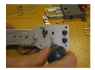
Tighten the retaining screws but DO NOT OVERTIGHTEN, the threads are into plastic spacers.
