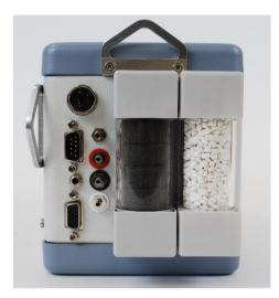
The LCi T is delivered with the internal battery fully charged and connected and the Soda Lime column filled with fresh self-indicating Soda Lime. This should be a pure, white colour.
