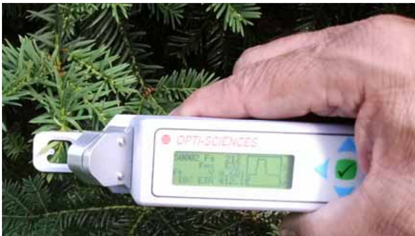
Page 1 of the measuring screen shows Y(II) , ETR, F_s , F_M' & the graph of Y(II)
