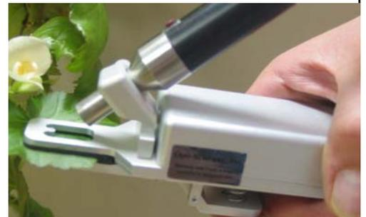
The Standard PAR Clip is designed for one hand operation. The underside opening mechanism prevents the weight of the fibre optic cable opening the PAR clip unexpectedly.
