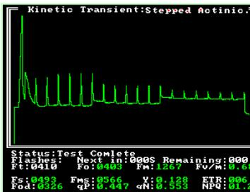
**Light curves:** Steady state photosynthesis at different levels of light intensity. Generation of light response curves using the unique OS5p ultra stable actinic light source. There is no requirement to use an external light source.
