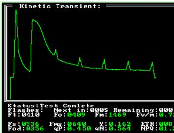
**Kinetic test:** Advanced quenching analysis using Puddle and Lake measuring parameters. Ultra stable light source ensures accurate measurements. NPQ, qP, qN and Y(II). Kramer lake model Y(II), Y(NPQ), Y(NO), Fod and qL Hendrickson lake model Y(II), Y(NPQ) Y(NO) and NPQ.
