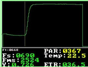
**Quantum Photosynthetic Yield Y(II):** Light adapted test allowing the measurement of PSII during photosynthesis. Sensitive for most types of plant stress. Reduces with stress. Improved accuracy of Y(II) using Fm' correction option for samples measured under high actinic light.
