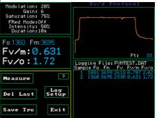
The most widely used fluorescence test requires pre-darkening of the leaf. The OS1p optimises Fv/Fm measurements by firstly automatically setting the modulated light source. Then secondly by providing a far red light option to ensure full oxidation of PSII prior to test.
