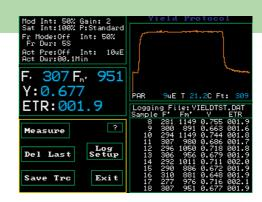
The OS1p can perform the most commonly used and widely respected fluorescence tests such as Fv/Fm, Photosynthetic Yield Y(II), ETR, NPQ and rapid light curve. The new Multi-flash test ensures reliable data even at high saturation light levels.
