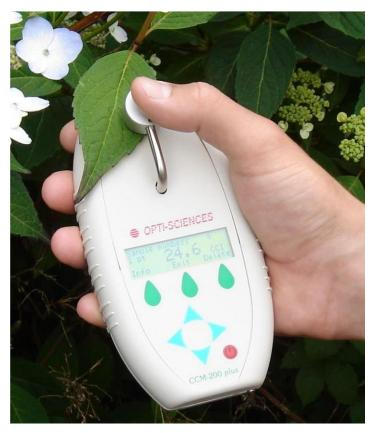
The *proven* **CCM-200***plus* provides fast and reliable chlorophyll content readings on intact plant leaves. The measurement is rapid, and easy to make with single hand operation. The instrument is especially useful for improving **Nitrogen** and **fertilizer** management programs with various crops such as corn and wheat. The CCM-200*plus* is used on a wide variety of both  $C_3$  and  $C_4$  plants.
